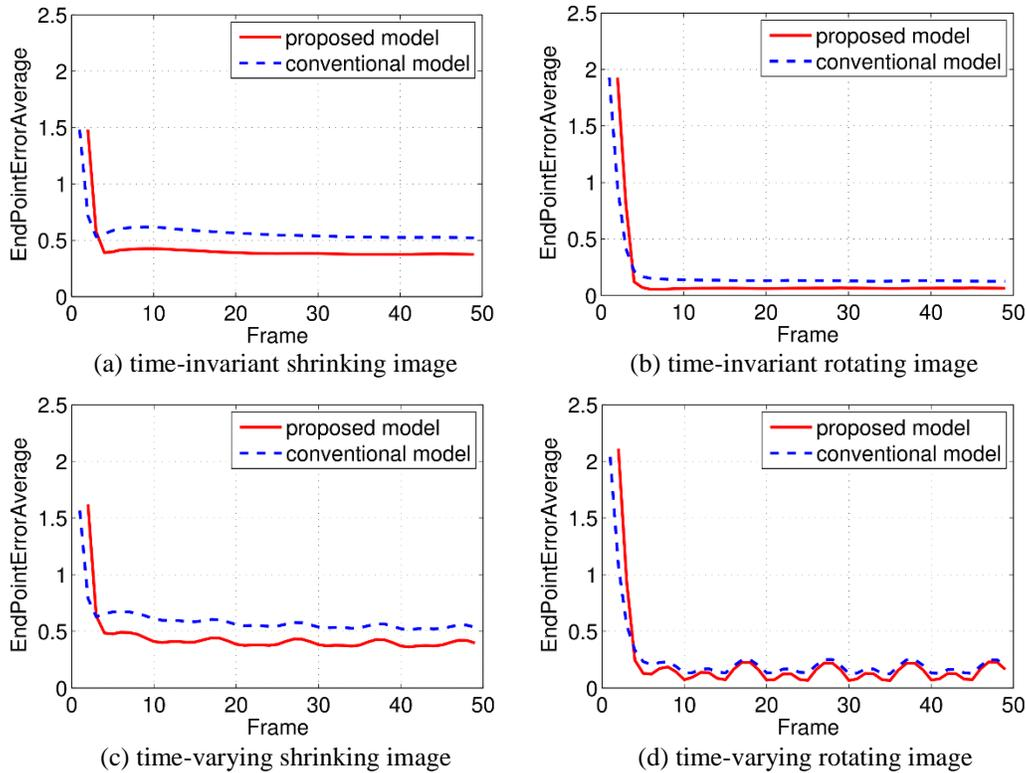
Fig. 2: Endpoint error average for each frame of the images.
