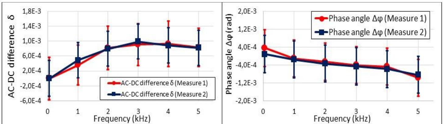
Fig. 4: AC-DC difference and phase angle at 2 A of the developed current shunt.
