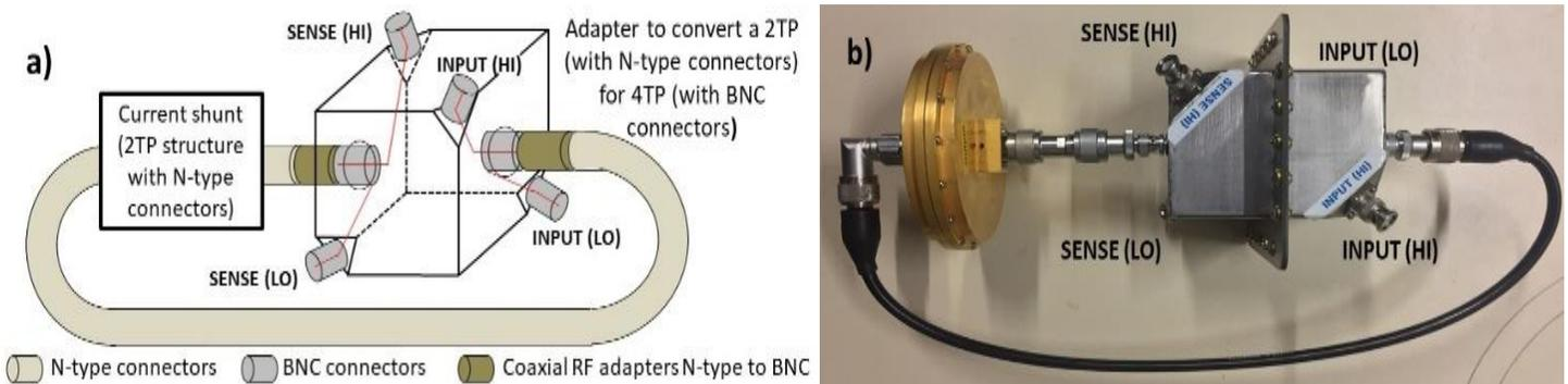
Fig. 3: a. Current shunt with the adapter box to convert a coaxial two terminal-pair device (with N-type connectors) in terminal-pair configuration (with BNC connectors). b. Final structure of the current shunt defined in four terminal-pair (with BNC connectors).
