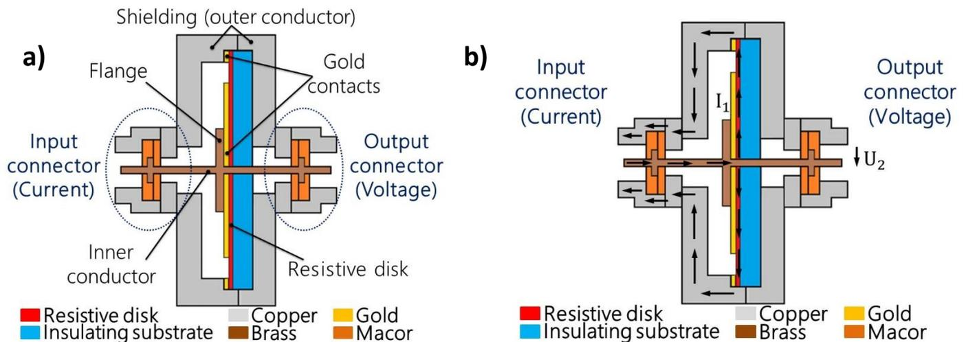
Fig. 1: a. Structure of the current shunt defined in two terminal-pair. b. Structure of the current shunt defined in two terminal-pair including input current and output voltage.
