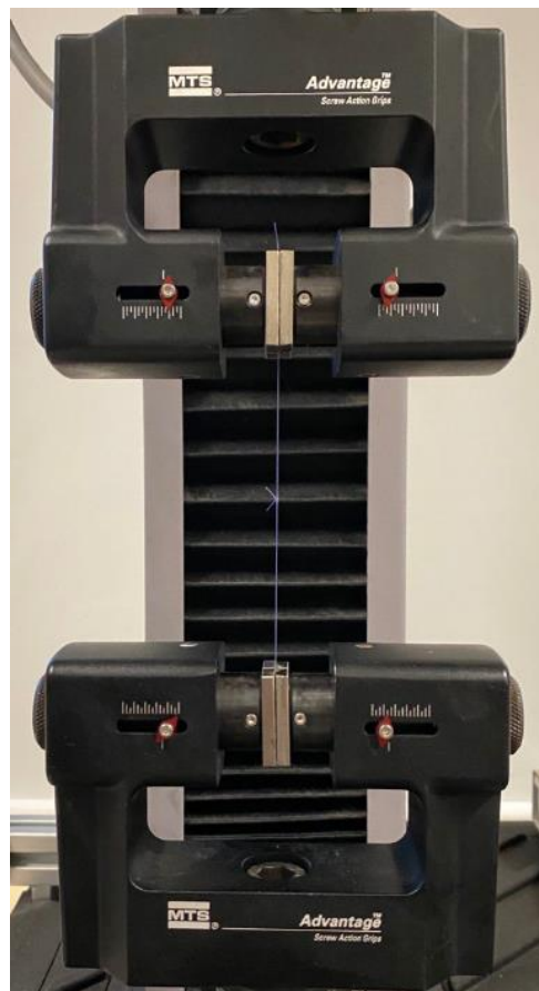
Fig. 3: Criterion 42 Universal tensile testing machine (MTS, Eden Prairie, MN) utilized in the mechanical testing phase
