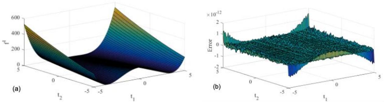
**Fig. 3.** Simulation results for  $f^1$ : (a) plot of function  $f^1$ ; (b) error between the function output and the SF model estimation.
