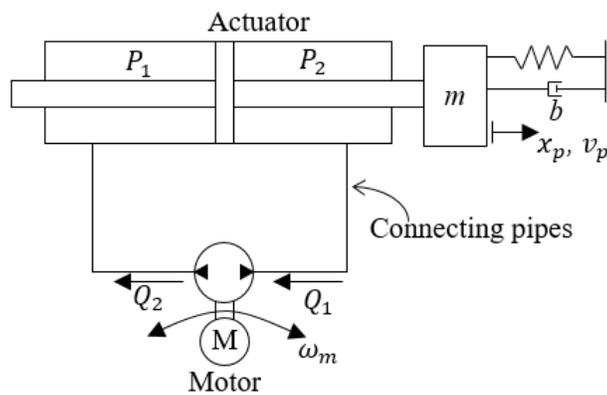
**Fig. 5.** Schematics of the electrohydraulic cylinder.
