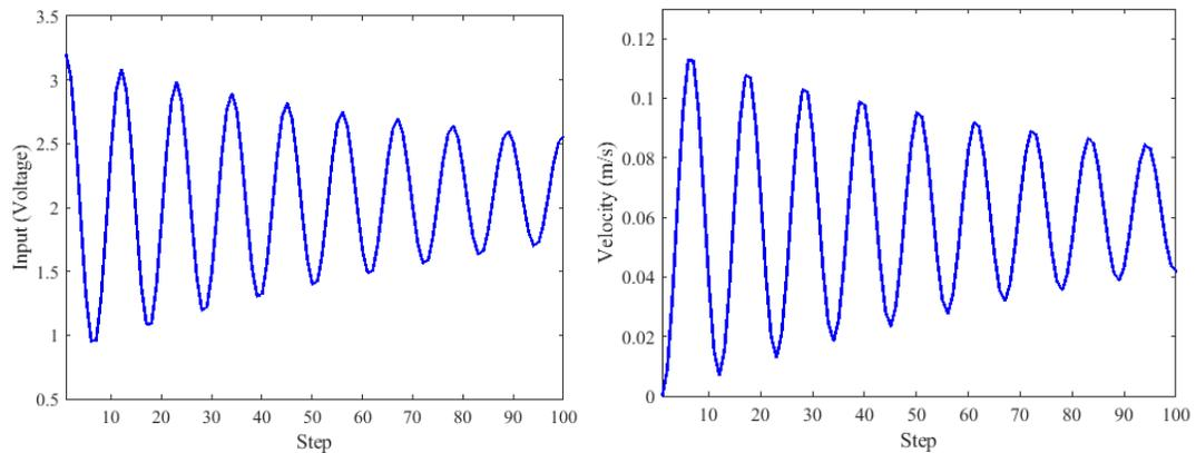
**Fig. 6.** Typical input and output (velocity) to the hydraulic system used for training.
