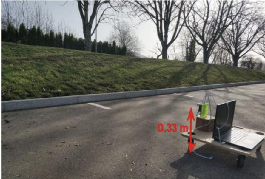
Fig. 7: Multipath based height estimation for curb at 2 m and 0.33 m sensor height.
