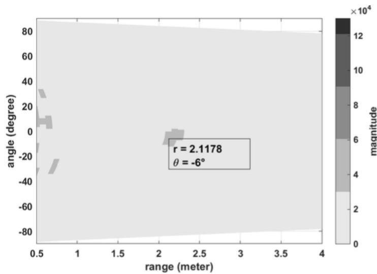
Fig. 3: AoA estimation for curb at 2 meters.
