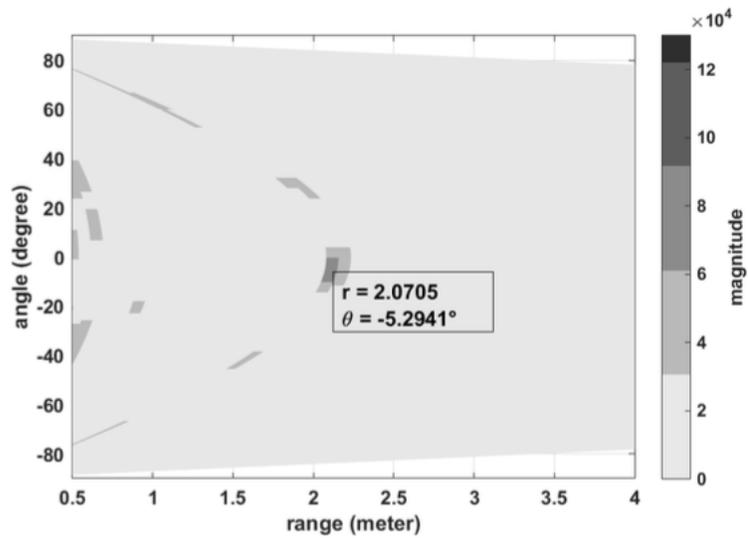
Fig. 2: AoA estimation for curb at 2 meters with AL.
