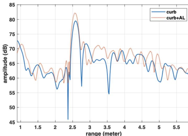
Fig. 5: Multipath based height estimation for curb at 2.5 meters with and without AL.
