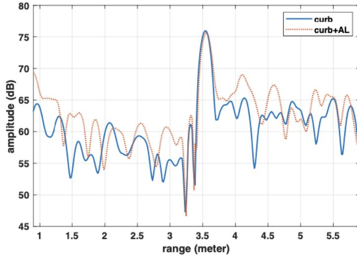
Fig. 6: Multipath based height estimation for curb at 3.5 meters with and without AL.
