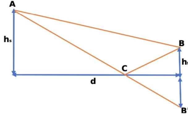
Fig. 4: A multipath propagation model. Propagation over a plane reflecting surface.
