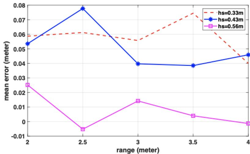
Fig. 8: Mean error of the estimated height for different radar heights from the multipath signal-based height finding algorithm.
