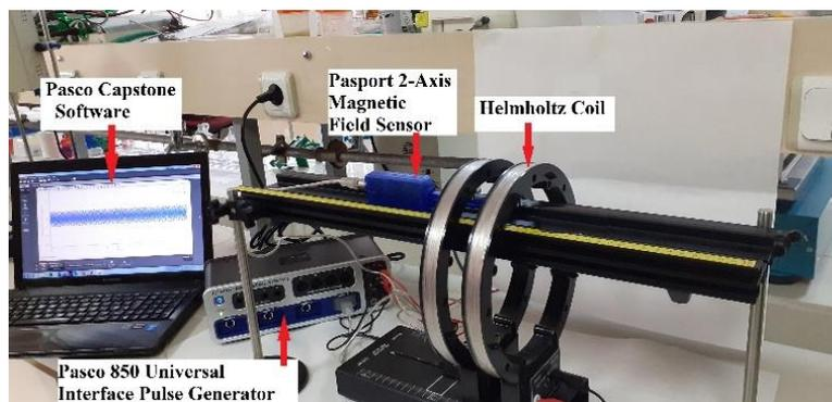
Fig. 1: Representative illustration of PEMF set-up with two-coil Helmholtz set-up.
