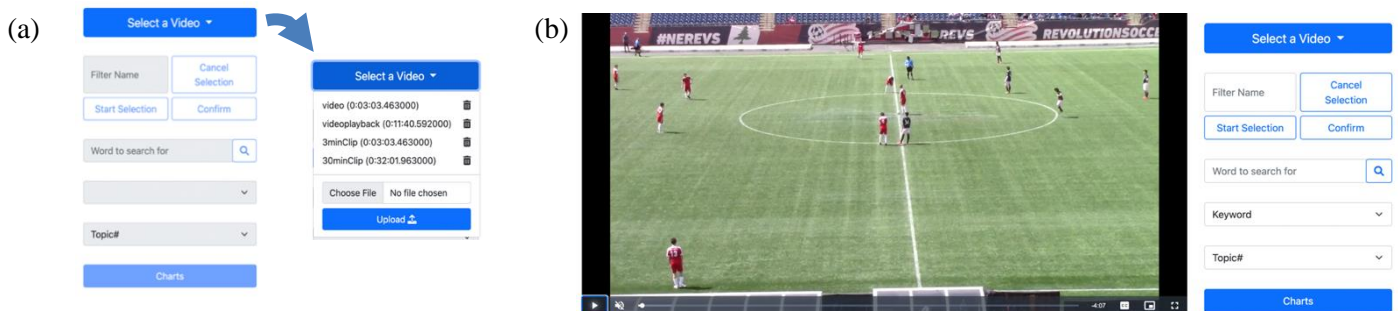
Fig. 1: (a) File selection dialogue: the user can either choose the videos that were previously analyzed or upload a new one. (b) Video player view: it provides typical video playback functions (on the left), as well as the video analysis controls (on the right).
