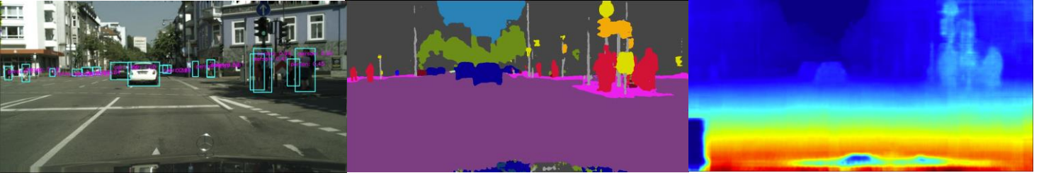
Fig. 2: Results of proposed network. Left: object detection, center: semantic segmentation, right: disparity estimation.
