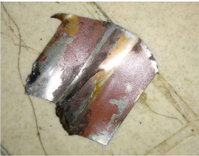
Fig. 5: Torn-out Piece of Lamination
