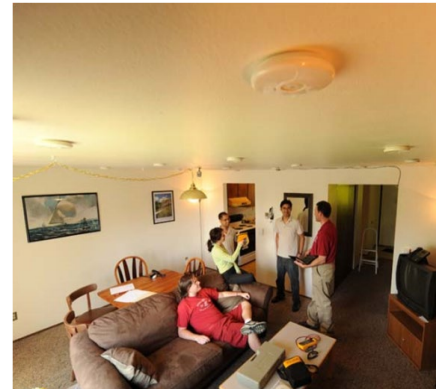
Fig. 1: CASAS motion sensors are placed on walls and ceilings; door sensors are placed on cabinets and exterior doors.
