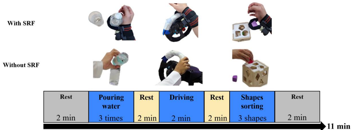
Fig. 2: Experiment design and setup including the two phases (with SRF and without SRF) and the three tasks (pouring water, driving, and shapes sorting).
