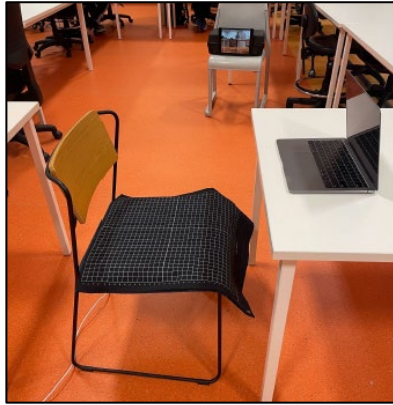
Fig. 1: CONFORMat setup on chair
