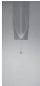
Figure 2 shows an example of good droplet formation.
