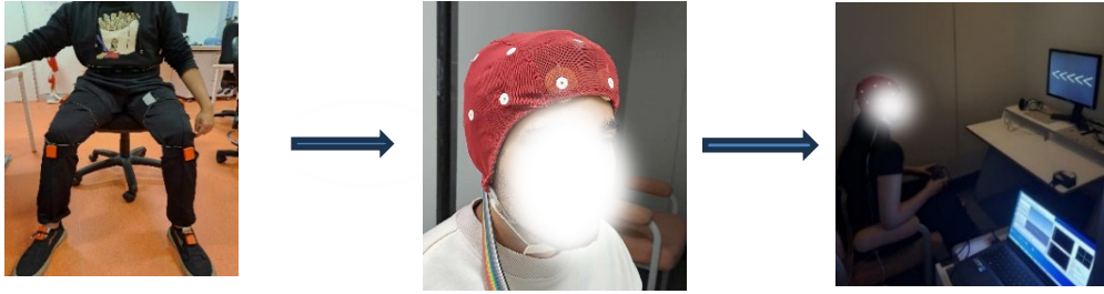
Figure 1: Xsens sensors on lower limb (Left), EEG Cap (Middle) & participant conducting the experiment (Right)
