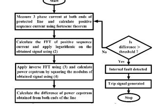
Fig. 1: Test bed for the power cepstrum scheme.
