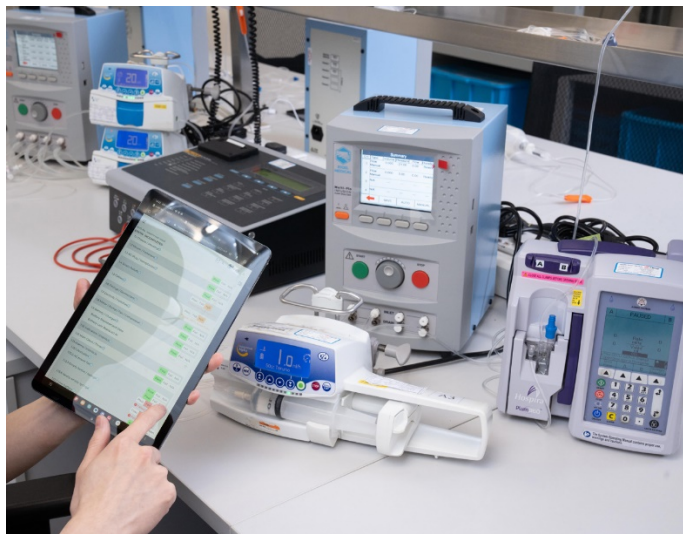
Fig. 2: Using BES eForm platform on tablet in centralized infusion pump maintenance line
