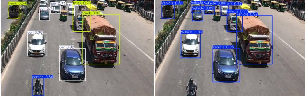
Fig. 4: YOLOv8 performance before (left) and after (right) fine-tuning on a vehicle dataset
