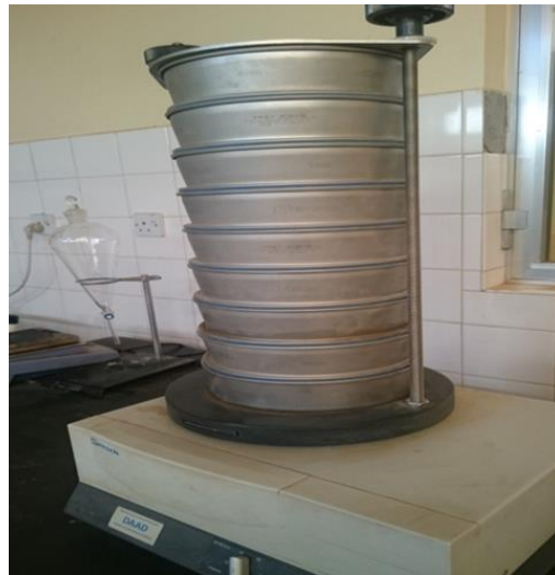
Figure 4. Vibrating Sieve to Sorting Dust Particles Size
