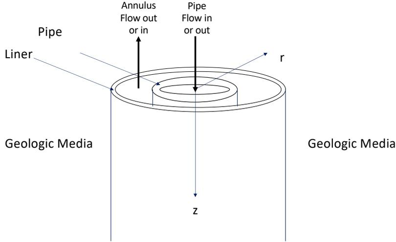
Figure 1. Configuration of the concentric wellbore configuration. The radial dimension is measured from the center of the pipe and  $z$  extends to the bottom of the wellbore. A liner (or large diameter pipe) is adjacent to the geologic media, with grout, if any, having the same thermal properties of the geologic media.
