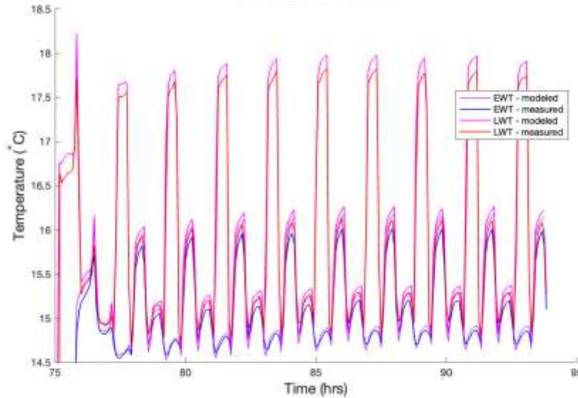
Figure 2. Detail of modeled heater inlet (EWT) and outlet (LWT) temperatures compared to data from cyclic heating (30 minutes of heating followed by 85 minutes heat off) from 75 hours to the end.
