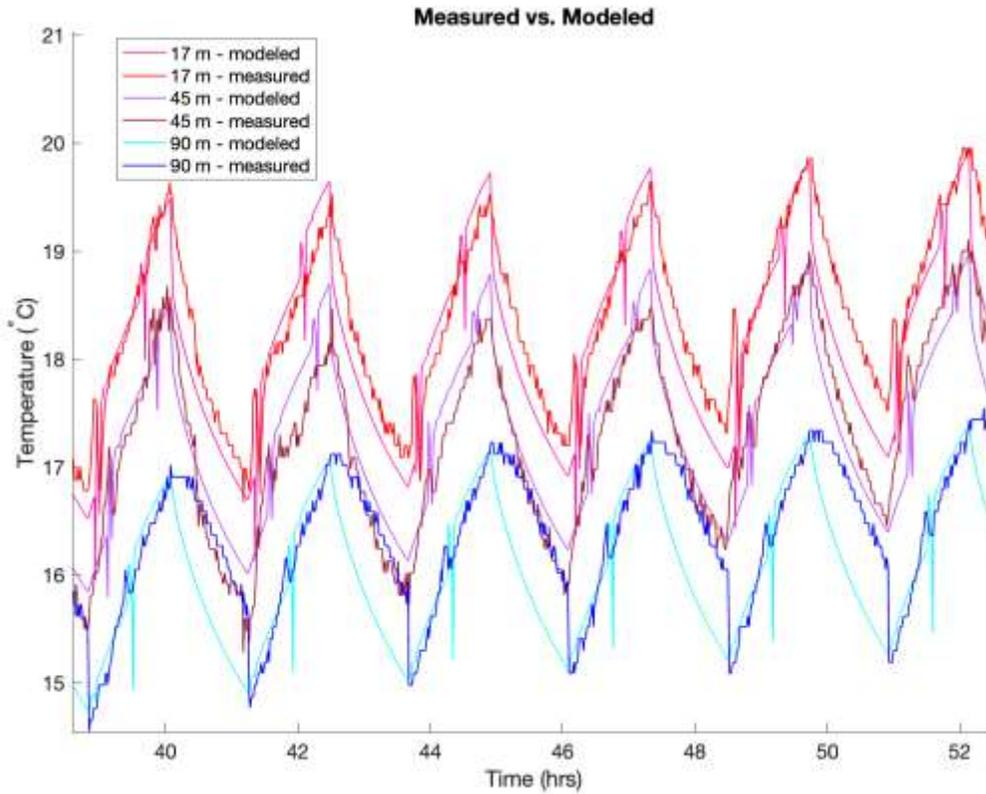
Figure 4. Detail of simulated and measured wellbore annulus temperatures, Test 3, annulus injection, cycling with 70 minutes on and 70 minutes off.
