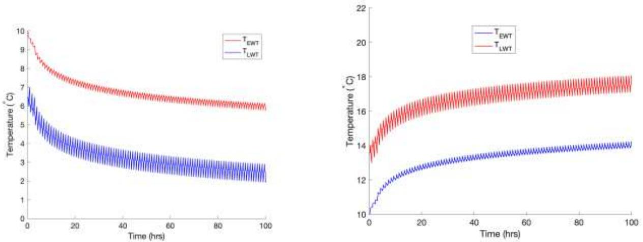
Figure 6.  $T_{EWT}$  and  $T_{LWT}$  for an 8" outside diameter borehole during heat pump operation, left, and refrigeration, right, of 20 minutes with heat transfer and pumping, and 40 minutes of rest.
