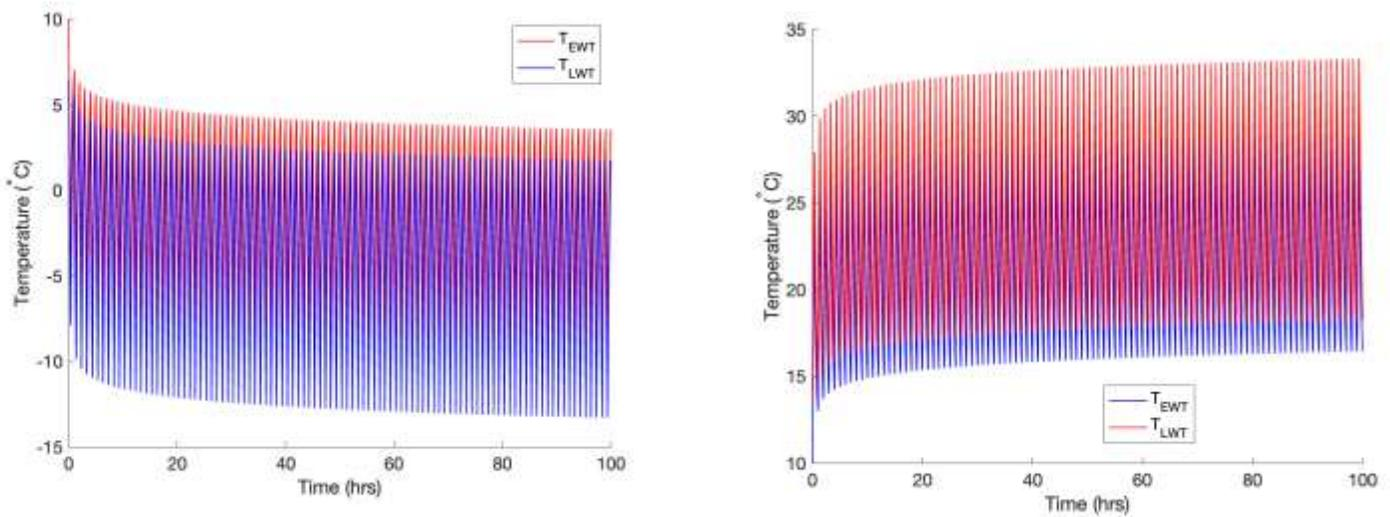
Figure 5.  $T_{EWT}$  and  $T_{LWT}$  for an 2" outside diameter borehole during heat pump operation, left, and refrigeration, right, of 20 minutes with heat transfer and pumping, and 40 minutes of rest.
