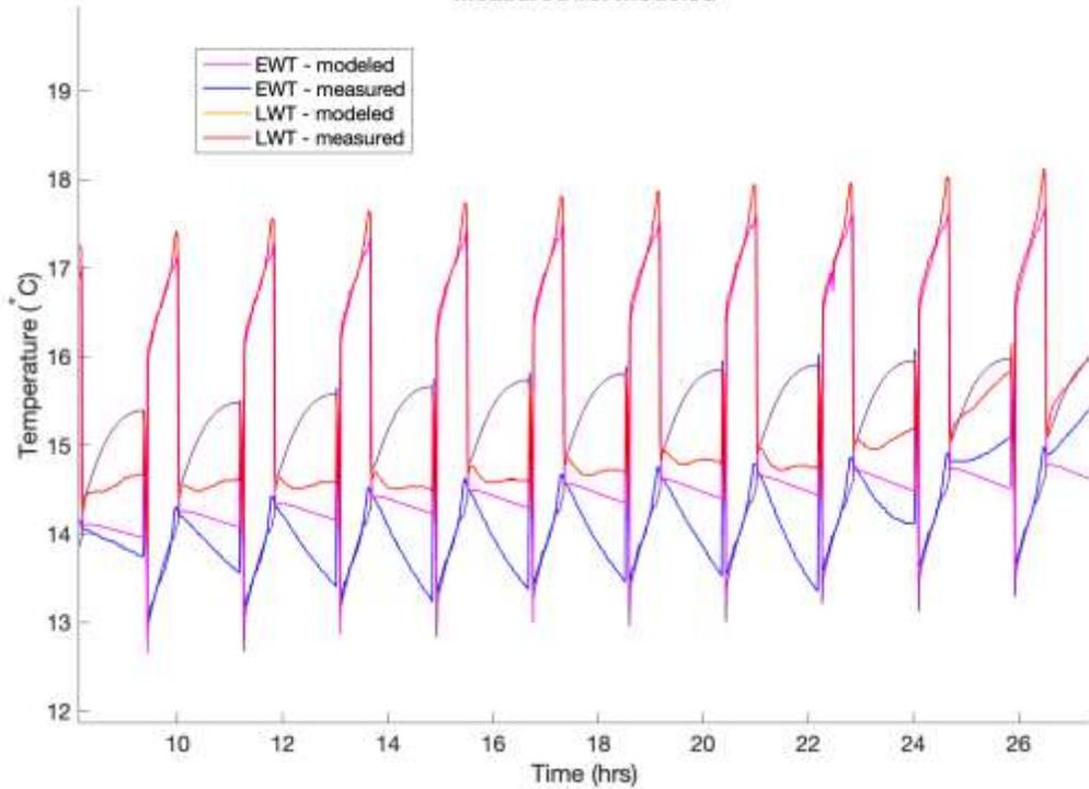
Figure 3. Detail of simulated and measured heater inlet (EWT) and outlet (LWT) temperature response during cyclic operation with a flowrate of 10.5 GPM, 8.8 kW heating for 35 minutes and resting for 70 minutes.
