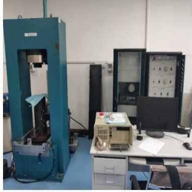
Fig. 1 TAW-2000 microcomputer-controlled electro-hydraulic servo rock triaxial testing machine.
