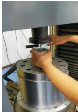
Fig. 3. Fixing the pore pressure reduction device on the rock triaxial testing machine
