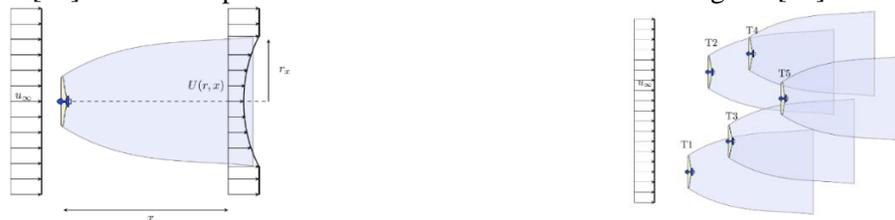
Fig. 2: Wake effect; left: single turbine wake effect, right: multi wake effect.
