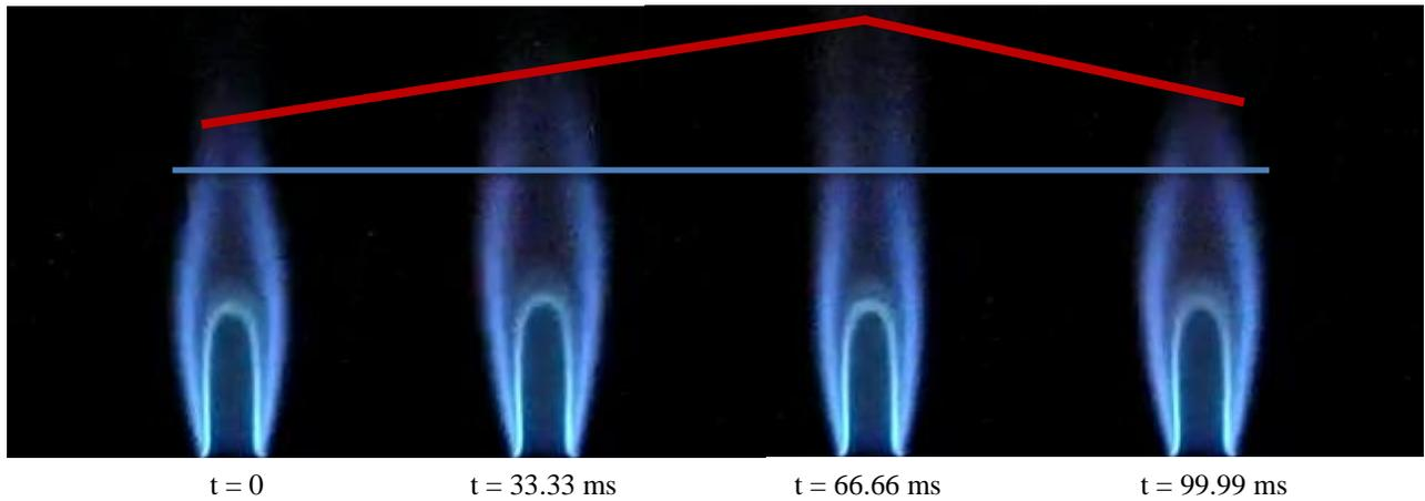
Fig. 5. Instantaneous Photographs of ER = 5.47 ( $Re = 135$ ,  $Fr = 26$ ) flame showing tip flickering mode of oscillation
