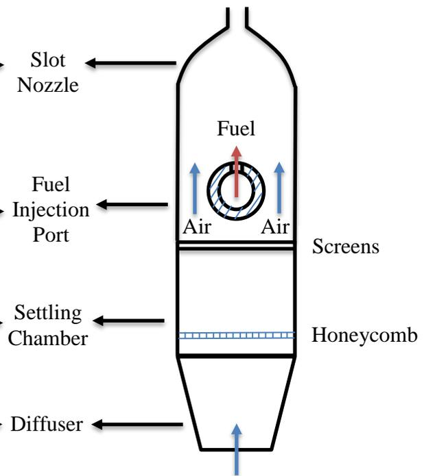
Fig. 2. Internal Geometry of Burner
