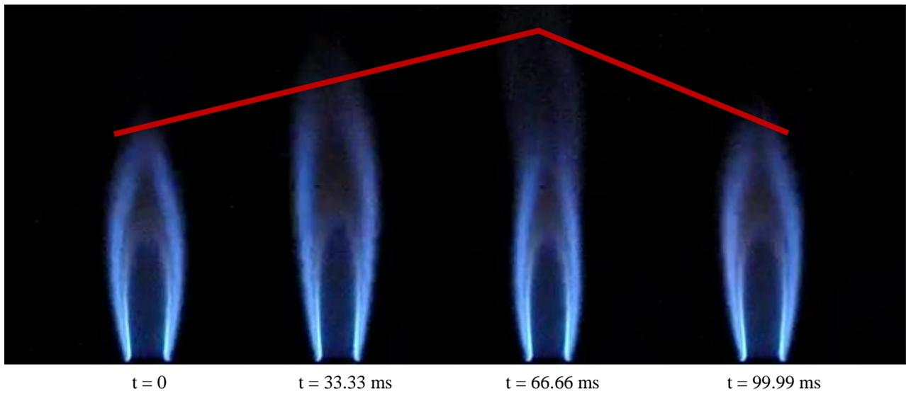
Fig. 4. Instantaneous Photographs of ER = 7.58 flame ( $Re = 106$ ,  $Fr = 16$ ) showing bulk flickering mode of oscillation
