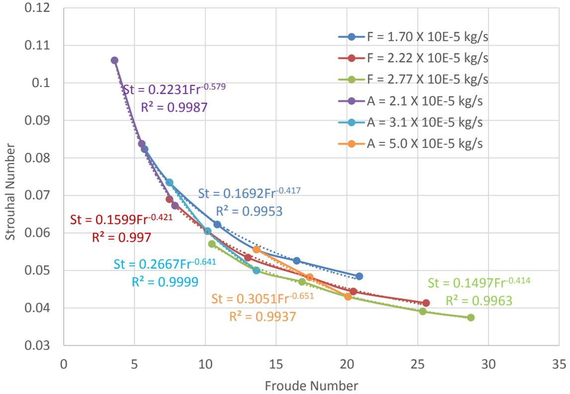
Fig. 7. Effect of air flow rate and fuel flow rate on  $St - Fr$  correlation for various fuel flow rates
