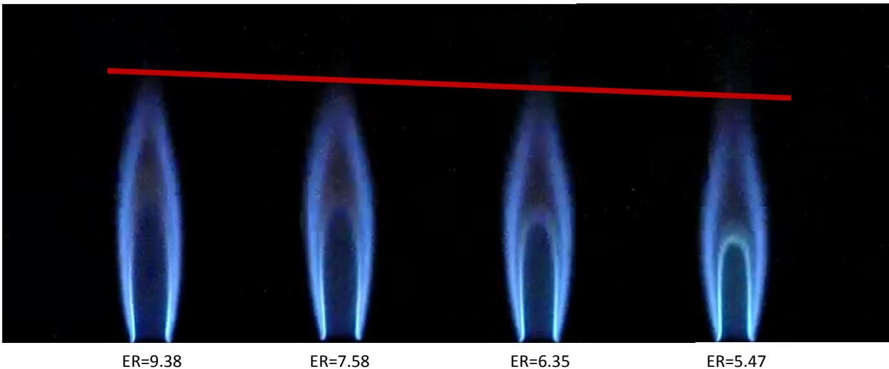
Fig. 3. Variation of flame height with partial premixing.  $Re$  varies from 91 to 135 and  $Fr$  varies from 13 to 26 as mentioned in the table 1.
