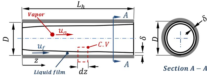
Fig. 1. Sketch of an annular flow model in horizontal circular channel
