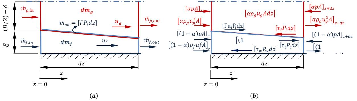
Fig. 2. A symmetric sketch shows basic terms for deriving: (a) mass conservation equation, (b) momentum equation
