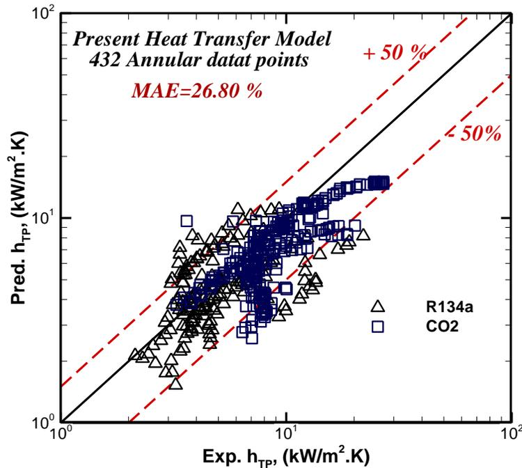
Fig. 1. Heat transfer coefficients predicted by the present model against those measured experimentally (423 data points) for various working fluids and operating conditions.
