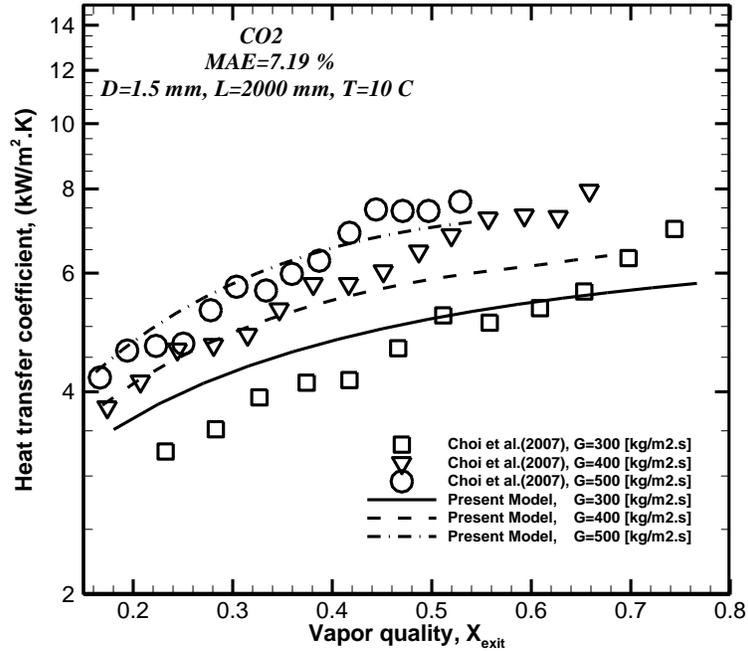
Fig. 3. Variation of heat transfer coefficient for flow boiling of the refrigerant CO<sub>2</sub> with exit vapor quality, and comparison with the experimental data of Choi et al. (2007).
