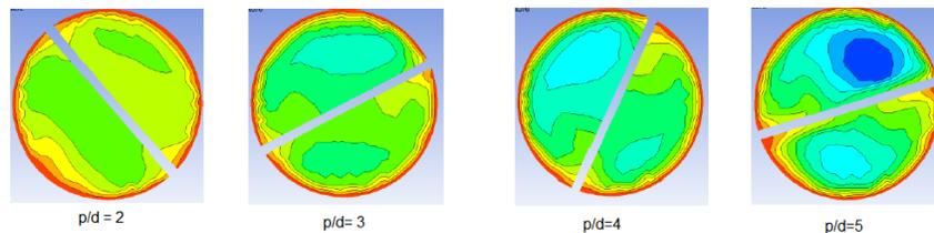
Fig. 7. Temperature contours for varying p/d at Re=800.
