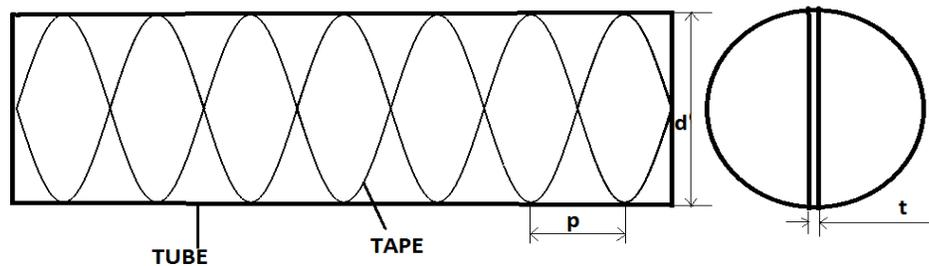
Fig. 1. Twisted Tape fitted inside tube.
