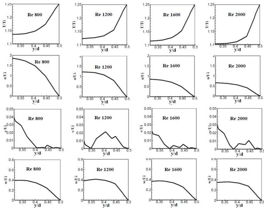
Fig. 9. Effect of varying Reynolds number on  $u$ -velocity,  $v$ -velocity,  $w$ -velocity and temperature near the wall.
