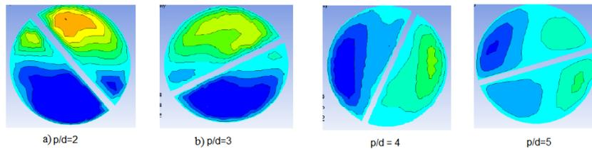
Fig. 6. W-velocity contours for varying p/d ratio at Re=800.
