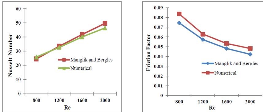
Fig. 2. Validation of numerically predicted Nusselt number and friction factor with those obtained by Manglik and Bergles for  $p/d=5$ .
