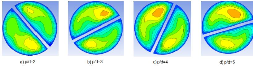
Fig. 4. U-velocity contours for varying p/d at Re=800.
