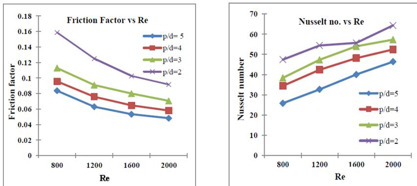
Fig. 3. a) Variation of Friction Factor and b) Nusselt number with Reynolds number.
