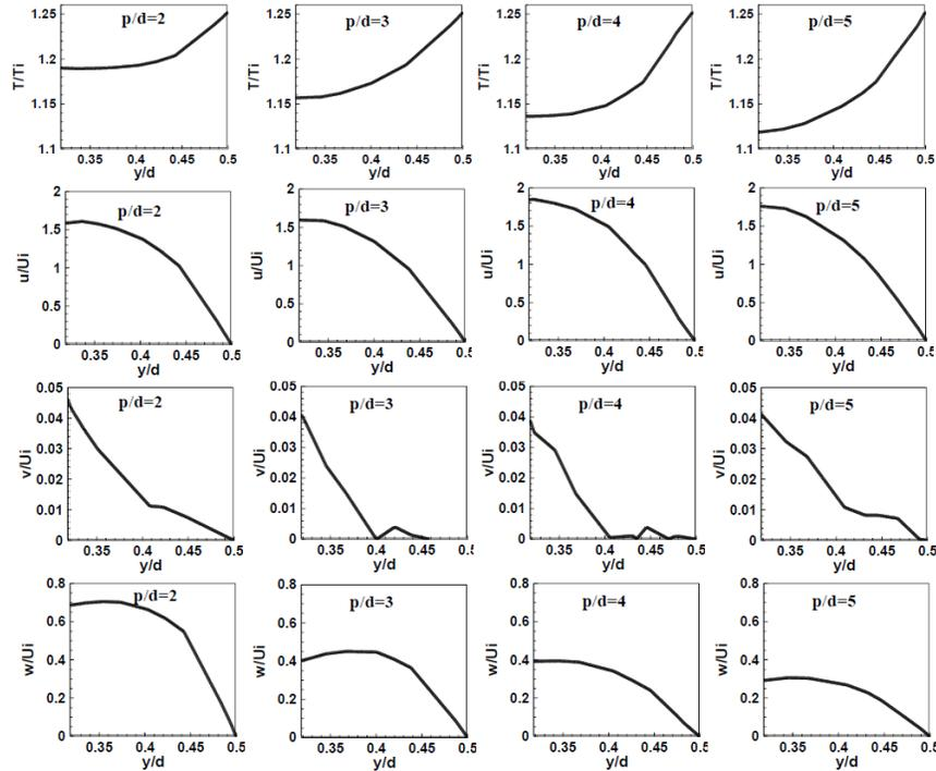
Fig. 8. Effect of variation of twist ratio on  $u$ -velocity,  $v$ -velocity,  $w$ -velocity and temperature near the wall.
