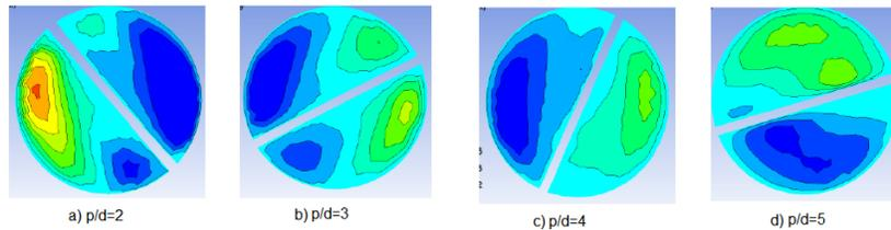
Fig. 5. V-velocity contours for varying p/d ratio at Re=800.
