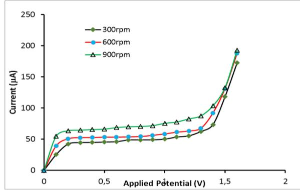
Fig. 3. Polarization Curves for different turbine rotational speeds.
