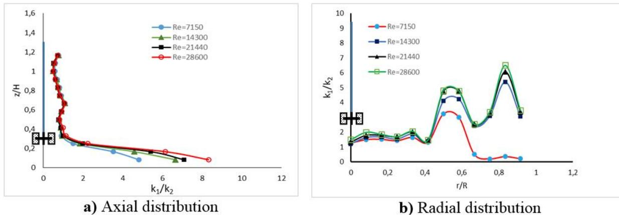
Fig. 4. Distribution of mass transfer coefficient ratio with nanopowder and no powder for ( $H/d$ )=1 and  $\theta=45^\circ$ .
