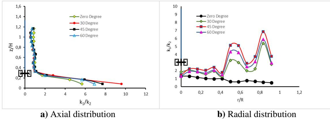
Fig. 5. Distribution of mass transfer coefficient ratio with nanopowder and no powder for  $Re=21440$  and  $(H/d)=1$ .
