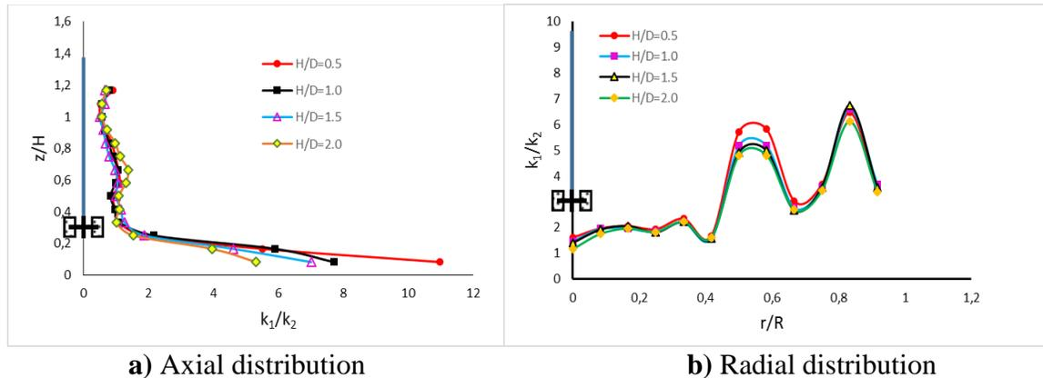
Fig. 6. Distribution of mass transfer coefficient ratio with nanopowder and no powder for  $Re=21440$  and  $\theta=45^\circ$ .
