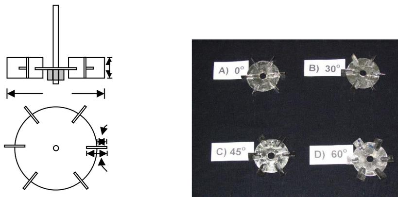
Fig. 2. Rushton turbine with four blades and the photographs used in the experiments.
