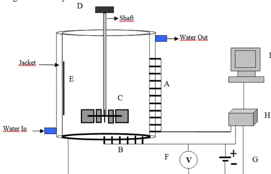
Fig. 1. The jacketted vessel agitated with Rushton turbine.
