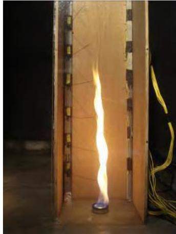
Fig. 5: Experimental footage of the fire whirl for 3.58 kW ethanol fire after Chow and Han [7].
