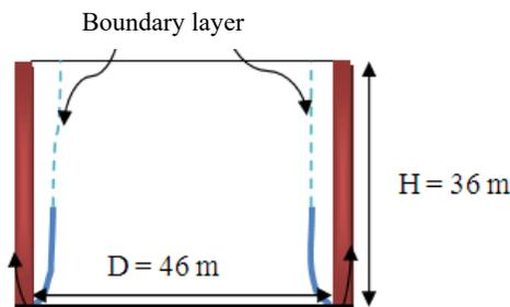
Fig. 1: Schematic of physical model for tank 37 000 m<sup>3</sup>.
