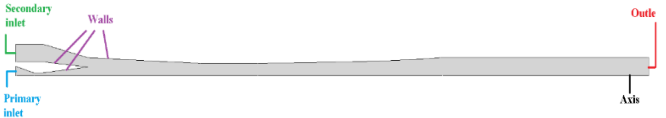
Fig. 3: Schematic of the ejector geometry and its boundary conditions.
