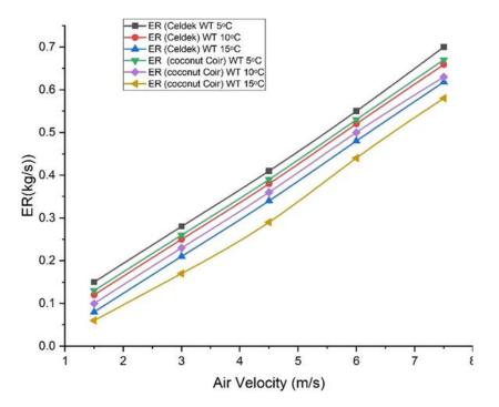
Fig. 6: Variation of evaporation rate with air velocity.
