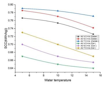
Fig. 9: Specific cooling capacity with water temperature.
