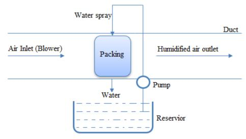
Fig.1: Principle of humidification.
