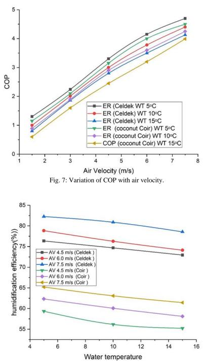
Fig. 8: Variation of Humidification efficiency with water temperature.
