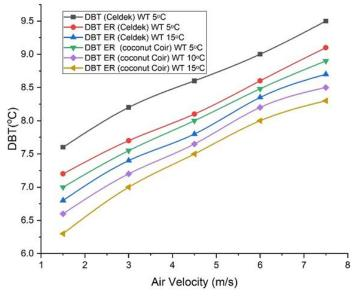
Fig. 10: Change in Dry bulb temperature with Air velocity.
