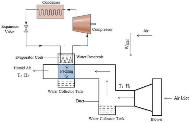
Fig. 2: Experimental set up for cross flow humidification.
