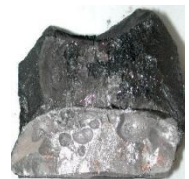
(e) cut of the post-mortem ingot of MA-3 test [6] – diameter is about 7cm
