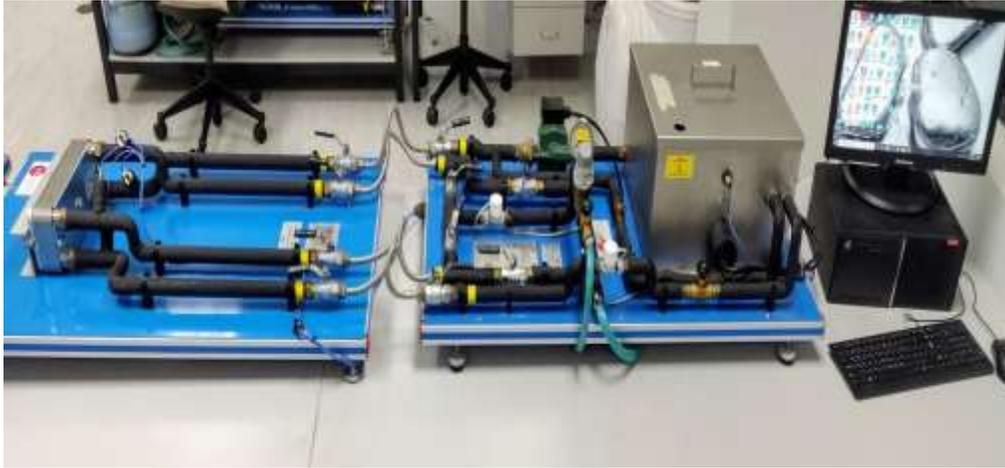
Figure 1: Plate heat exchanger experimental facility
