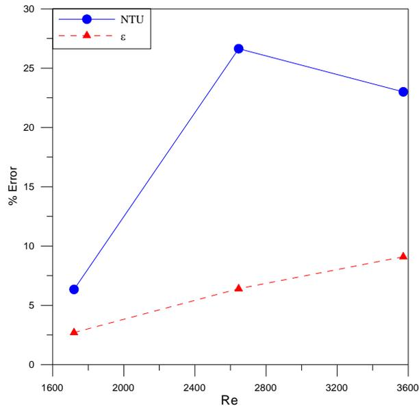
Figure 4: Deviation in NTU value and effectiveness predicted by the two models at different nanofluid flowrate
