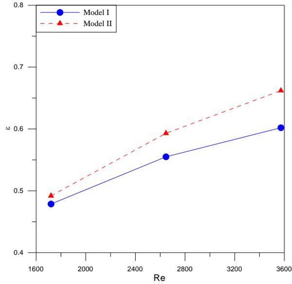
Figure 3: Comparison of exchanger effectiveness predicted by Model-I and Model-II
