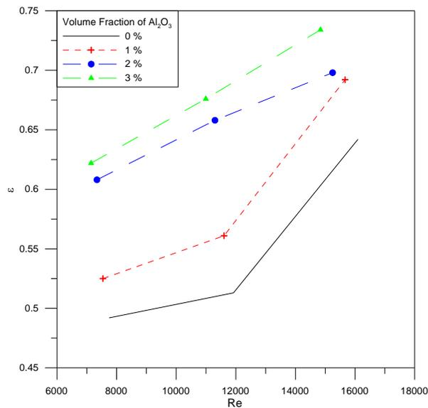
Figure 6: Exchanger performance against Reynolds number at different volume fractions of  $\text{Al}_2\text{O}_3$
