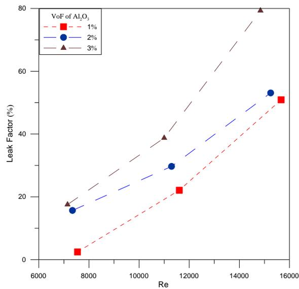
Figure 8: Heat leak factor versus Reynolds number at various fractions of  $\text{Al}_2\text{O}_3$
