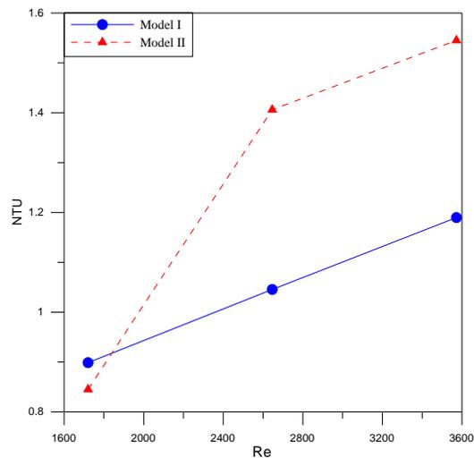
Figure 2: Comparison of exchanger NTU predicted by Model-I and Model-II
