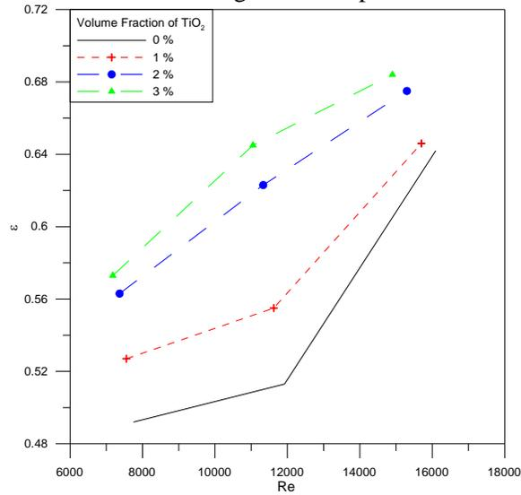
Figure 5: Exchanger performance against Reynolds number at different volume fractions of  $\text{TiO}_2$
