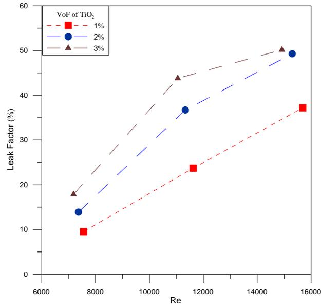
Figure 7: Heat leak factor versus Reynolds number at various fractions of  $\text{TiO}_2$
