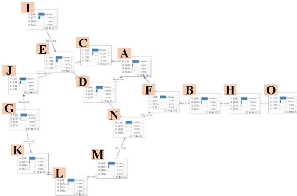
Fig. 1. BBN structure for the mean tke subdomain field based on the application of the PC algorithm. Multidimensional scaling format is shown. Horizontal plane subdomains are labeled with letters. Arrow thickness parameterize the strength of edge connections.
