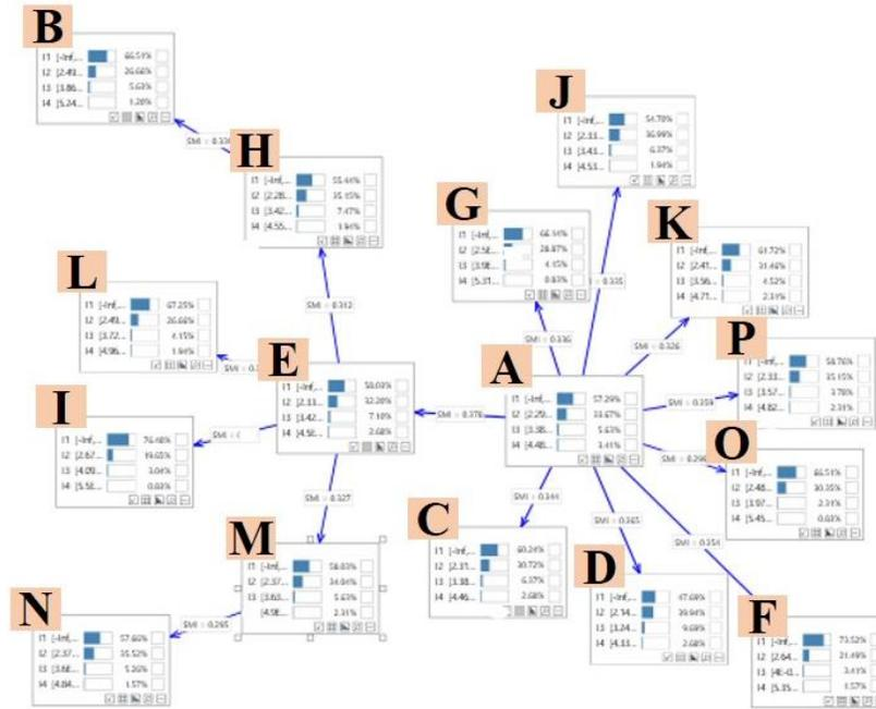
Fig. 2. BBN structure for the mean tke subdomain field based on the application of the Chow-Liu algorithm. Multidimensional scaling format is shown. Horizontal plane subdomains are labeled with letters. Arrow thickness parameterize the strength of edge connections.
