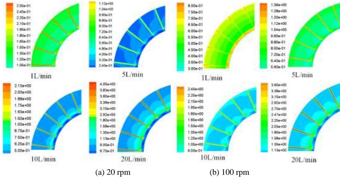
Fig.5: Lubricating oil flow field rate distribution
