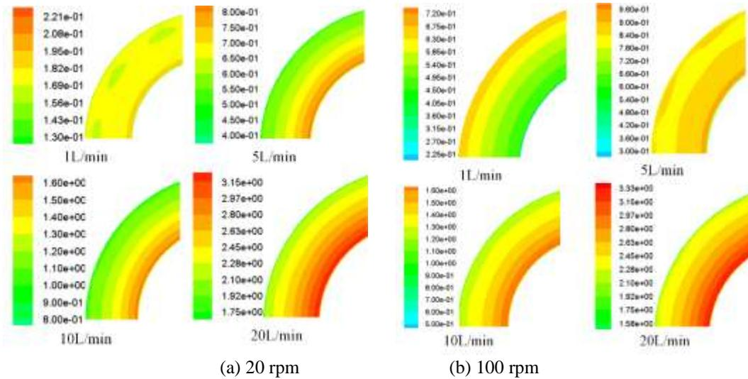
Fig.3: Lubricating oil flow field rate distribution
