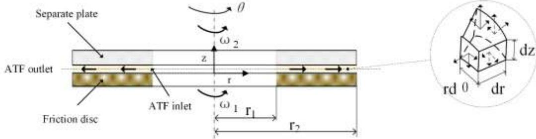
Fig. 1: Wet friction pair model.
