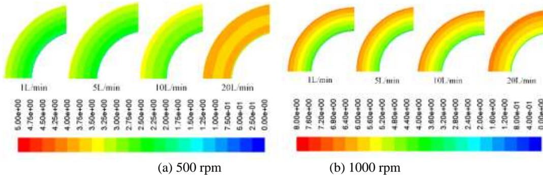
Fig.4: Lubricating oil flow field rate distribution
