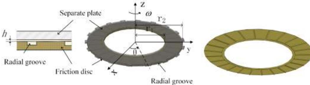
(a) Friction disc with radial grooves (b) Lubricating oil model
