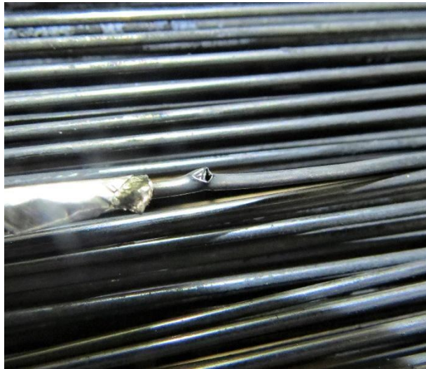
Fig. 3: Detail of defect on polyamide hollow fiber
