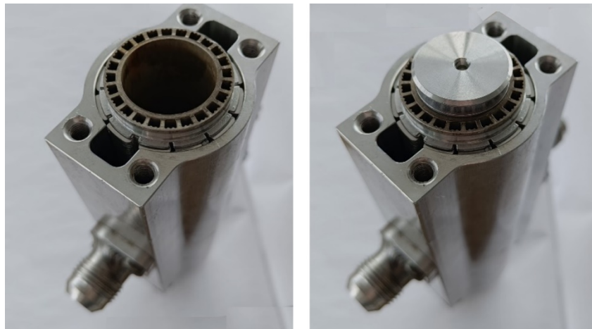
Figure 6: A unbaffled (left picture) and an baffled (right picture) arrangement of oil cooler.
