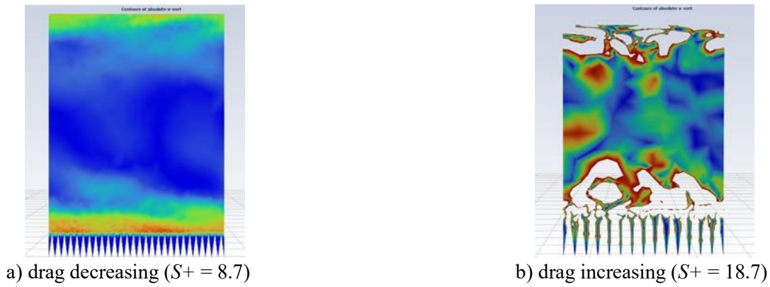
Fig. 7: Contours of streamwise vorticity for: a) \alpha = 15^\circ drag decreasing ( S^+ = 8.7 ) and b) \alpha = 15^\circ drag increasing ( S^+ = 18.7 ) cases.
