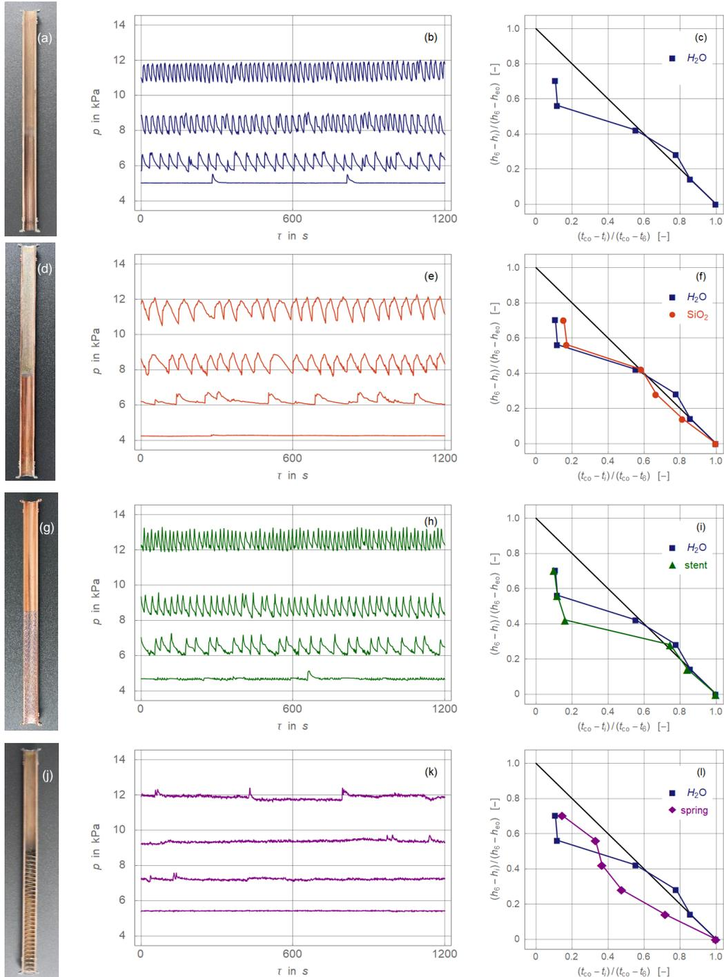
Fig. 2: Thermosyphon experimental results at  $t_{ci} = 15^\circ\text{C}$ . The left column presents the copper tubes cut after each experimental series.
