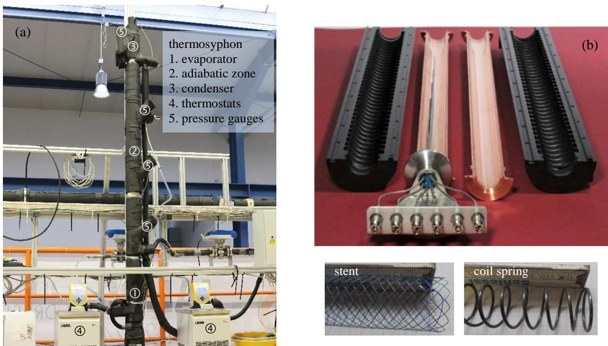
Fig. 1: Thermosyphon test rig. The insulated thermosyphon (a) consisting of the evaporator (400 mm), the adiabatic section (1,000 mm), and the condenser (400 mm). Image (b) presents the open evaporator. The black shells enclose the evaporator tube (copper) and guide the heating water flow. The temperature probe lays in the left evaporator tube half. The stent and the coil spring are inserted into the copper pipe to modify the boiling zone.
