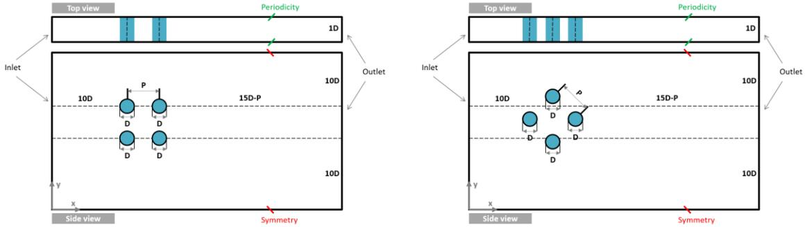
Fig. 2: Computational domain of four cylinders in a square arrangement with pitch to diameter ratio  $P/D = 1.5$ . (a) in-line configuration, (b) staggered configuration.
