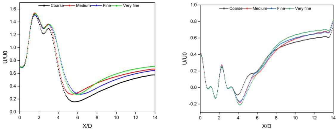
Fig. 4: Sensitivity study for the mean velocity along the centerline ( $Y/D = 0$ ).
