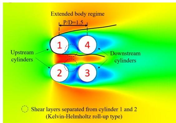
Fig. 6: The extended body regime for  $P/D = 1.5$  showing the shear layers that separate from the upstream cylinders wrap around the downstream cylinders.
