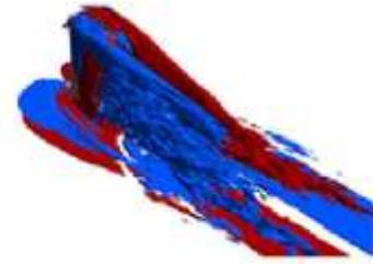
Fig. 11. Downwash flow and trailing edge vortices behind of the cylinder
