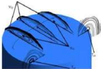
Fig. 9 Separated bubble and tip vortex formation at top free end
