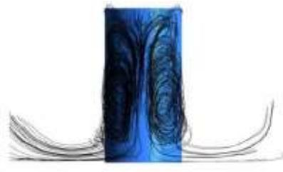
Fig. 10. Arc vortex behind the cylinder
