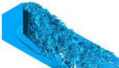
Fig. 6: Unsteady separated flow at top of the cylinder and downwash wake region behind the cylinder.
