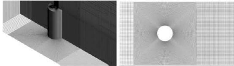
Fig. 3. Computational grid over the finite circular cylinder
