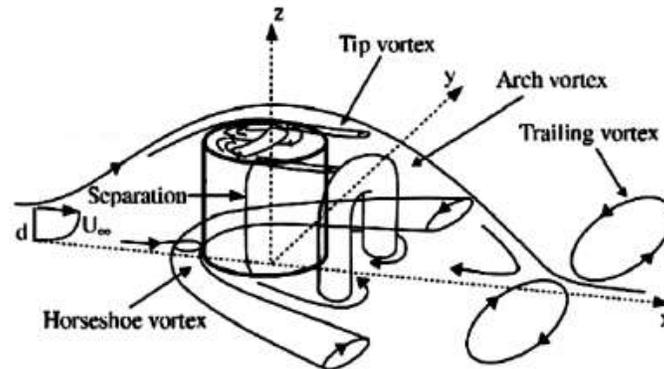
Fig. 1. Sketch of flow structure around the finite circular cylinder (Agui and Andreopoulos 1992).
