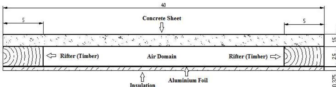
Fig. 1. Physical domain and dimensions (cm) of the roof.
