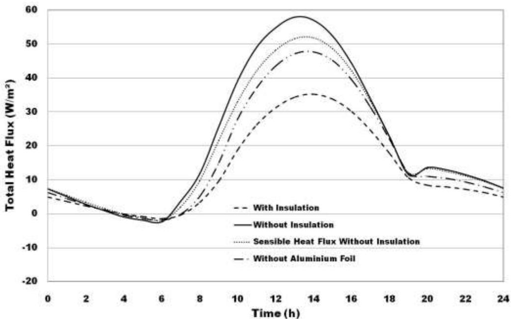
Fig. 2. Heat fluxes at the internal roof surface.
