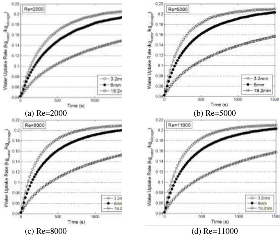
Fig. 4. Water uptake rate for different honeycomb cell size.
