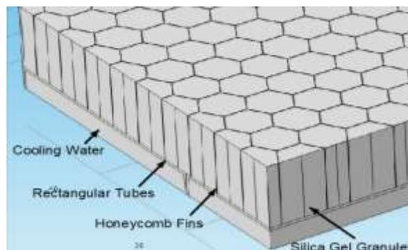
Fig. 1. Diagram for one quarter of adsorption bed.
