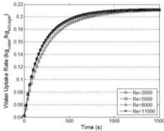
Fig. 5. Water uptake rate for different cooling water flow rates.
