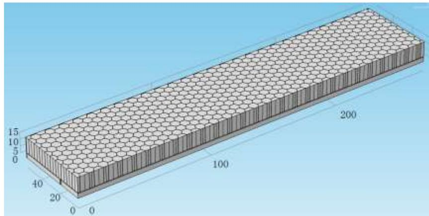
Fig. 2. COMSOL model of quarter of the adsorption bed.
