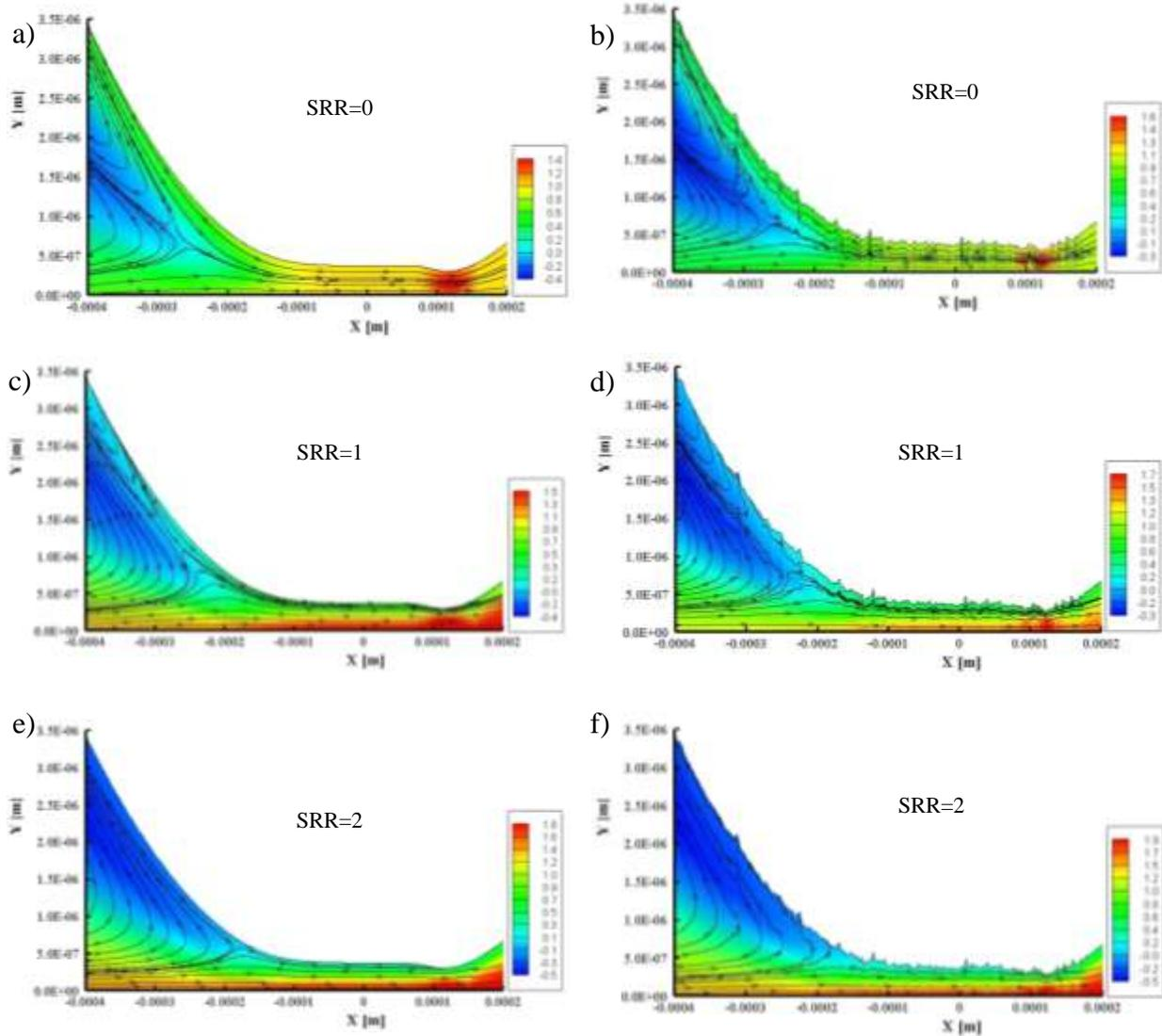
Fig. 5. Comparison of the velocity (m/s) between the smooth surface (left) and the rough surface (right) case at SRR=0, 1 and 2
