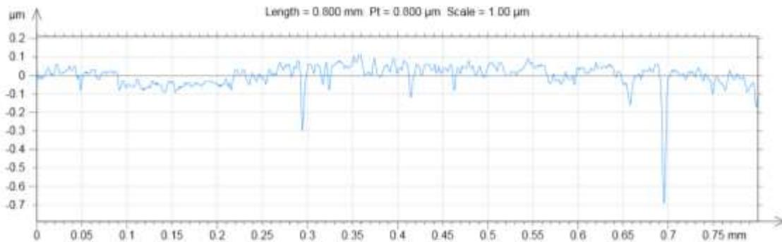
Fig. 2. A sample of the real rough profile on the cylindrical roller bearing.
