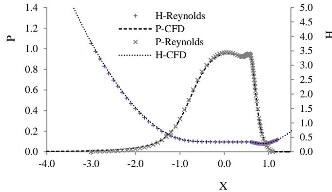
Fig. 3. Comparison of dimensionless pressure distribution and film thickness between the CFD model and the Reynolds equation.
