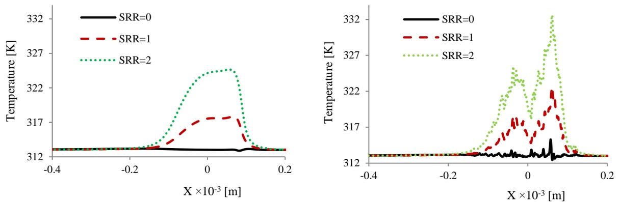
Fig. 6. Comparison of temperature distribution on the surface of cylinder between the case of smooth surface (left) and the rough surface (right) at SRR=0, 1 and 2.
