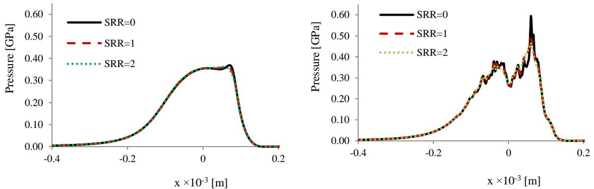
Fig. 4. Comparison of the pressure distribution between smooth surface (left) and rough surface (right) cases at SRR=0, 1 and 2
