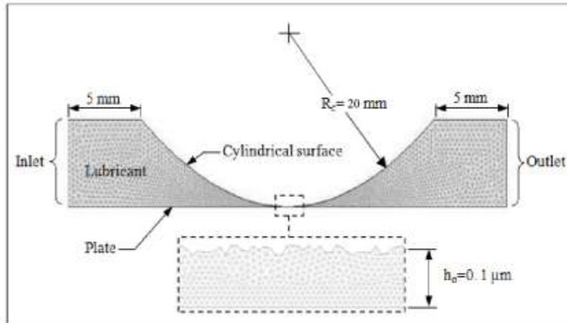
Fig. 1. The CFD model of the EHL problem with surface roughness.
