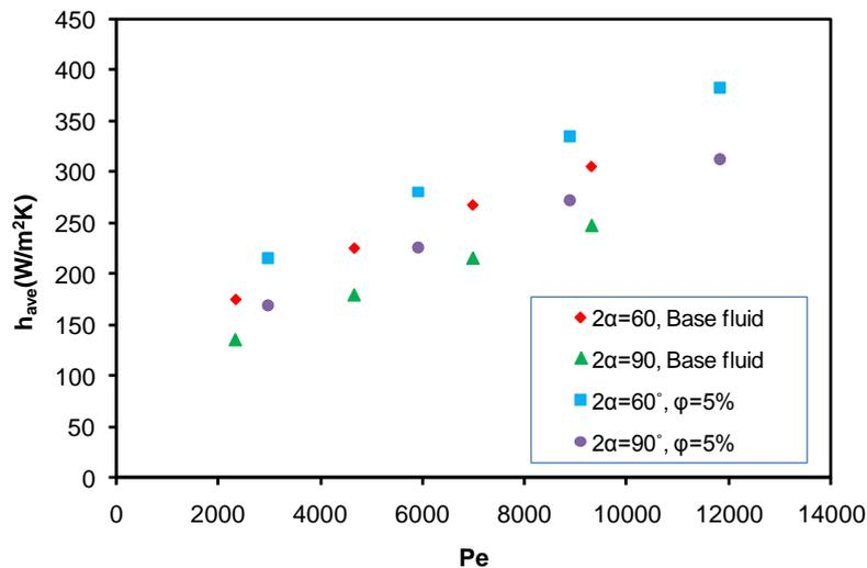
Fig. 4. Average heat transfer coefficient of nanofluids vs. Pe for different values of channel apex angle and different nanoparticle concentrations
