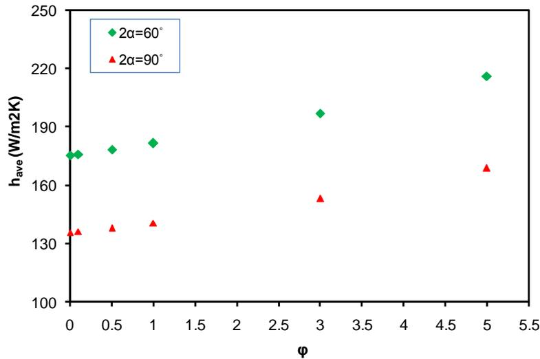
Fig. 5. Average heat transfer coefficient of nanofluids vs. nanoparticle concentration for channels with different apex angles.
