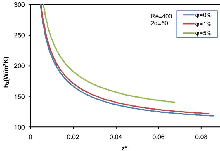
Fig. 3. Local heat transfer coefficient of nanofluids vs. axial position for different nanoparticle concentrations.
