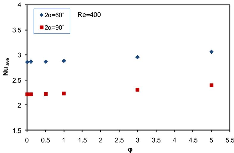
Fig. 6. Average Nusselt number vs. nanoparticle concentration for channels with different apex angles.
