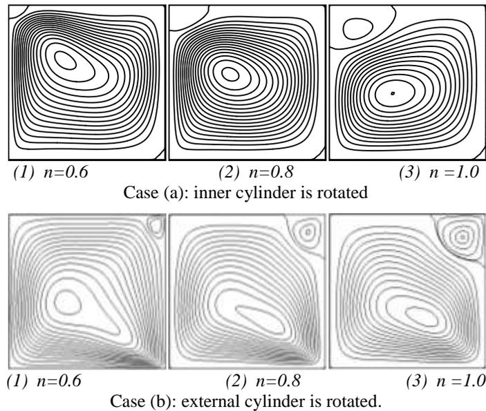
Fig. 4. Streamlines at  $Gr=2000$
