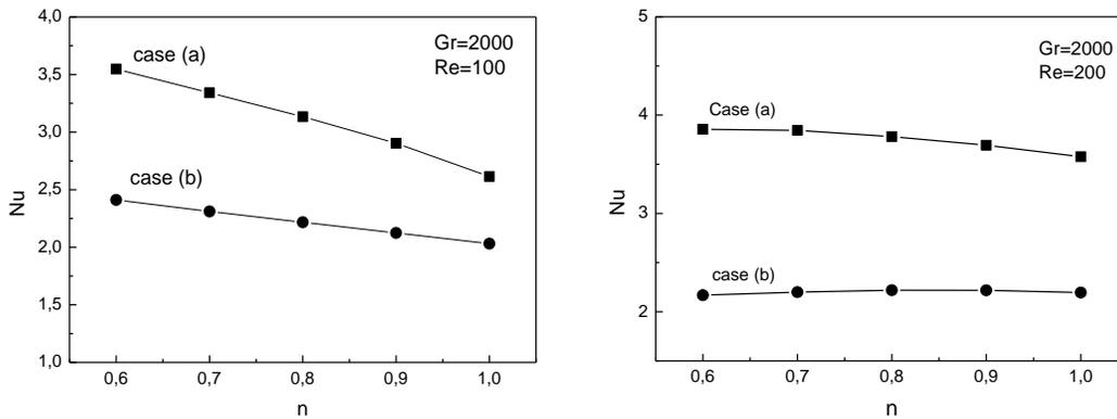
Fig. 2. Average Nusselt number as a function of the flow index at  $Re=100$  and  $Re=200$  for two cases.
