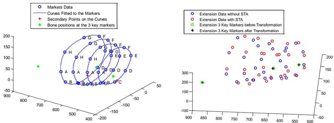
Fig. 6. Curve Fitting to Motion Capture Data and Determination of Bone Positions at 3 Key Points Positions of Standing Position (left), Transformation of Standing Markers to Extension Movement (right).
