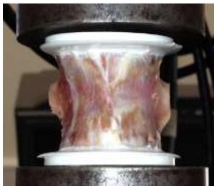
Fig. 2. Specimen for uniaxial compression testing of porcine vertebra body.
