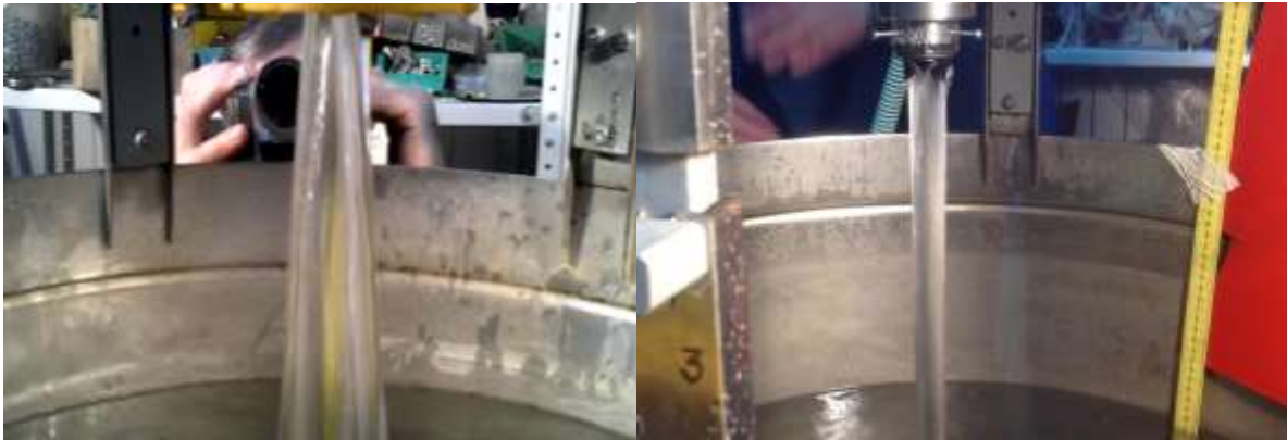
Fig. 4. The degree of Tornado-like jet conservation after Bicuspid (MEDENG)(left) and TCV (right) mechanical valve prostheses.
