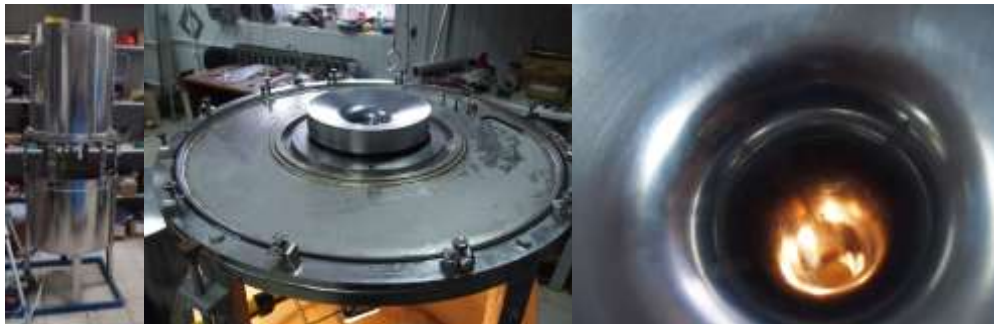
Fig. 2. Hydrodynamic stand for valve testing in the free-falling jet (left), converging channel for Tornado-like jet generating fitted in the bottom of upper tank (middle), the lumen of converging channel (right).
