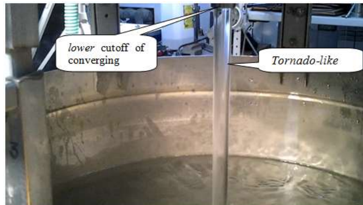
Fig. 3. "Glass" transparent jet, obtained on the outlet of converged channel.
