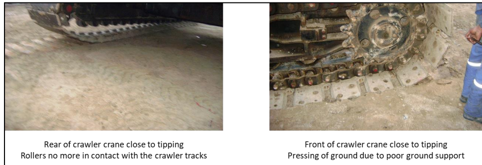
Fig. 1: Crane tipping due to poor ground support.
