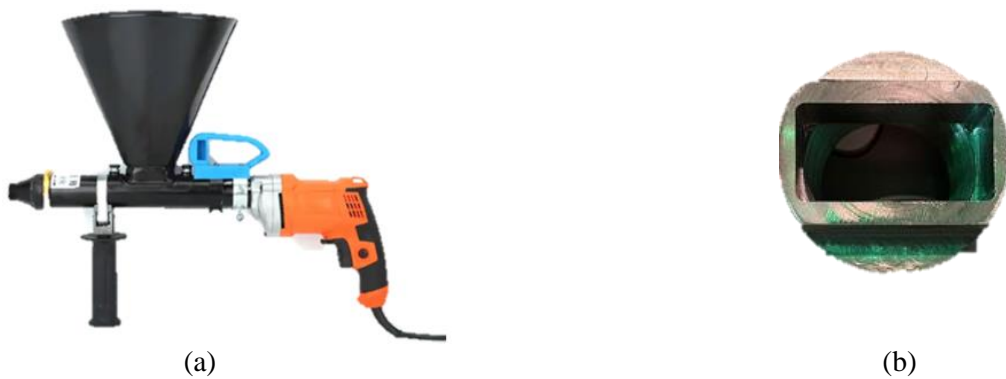
Fig. 1: (a) Mortar filling device; and (b) Front view of the nozzle.
