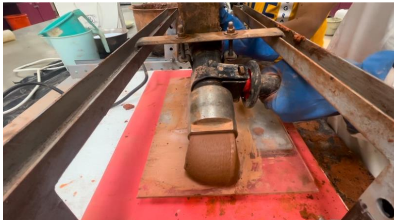
Fig. 2: 3D printing of the first layer using the developed printer.
