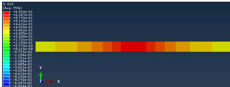
Fig. 4. Cross-sectional contour for shear  $S_{23}$  at  $z=147.8\text{mm}$  (reference Case R1) (Length scale factor for  $Y$  dimension =7)
